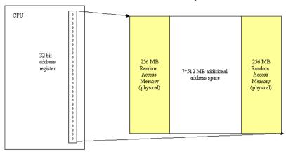
A 32-bit CPU can address 4GB of RAM. Most machines do not have so much physical memory. Notice that physical memory can be at several location in the overall addressable space. It is even possible to have systems with more memory than addressing capabilities. In those cases "bank switching" is used to allow the CPU to address different memory regions over time
