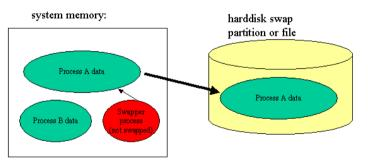
An operating system can swap out complete processes if the system memory is all used up. It will usually pick large processes for this and wait to swap them back in for some time to avoid thrashing. Before paging most OS used this mechanism which is more of a last resort nowadays. Text need not be stored because it can be reloaded from disk easily. A system process called "swapper" selects processes for swapping.
