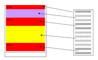
A bitmap is a fast and compact way of storing metadata about a large number of resources. If a new process needs to be created the memory manager must walk through the bitmap to find a piece of 0's large enough to fit the process in. This can take a while.
