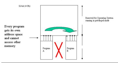
The price of separate program memory areas is that user programs which want send or receive data from other programs must do so via kernel interfaces (system calls). This is not cheap as data need to be copied back and forth from user space to kernel and from kernel to user space. (We will consider context switching times in our lecture on processes and concurrency)
