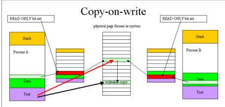
During process creation parent and child process share addess spaces. To prevent data corruption the OS sets the READ ONLY bits in the page table entries. If a process tries a write a page fault happens which makes the OS allocate a new physical frame as a writeable copy of the shared frame. From then on both processes have writeable frames. Instead of copying page frames for the new process only the page table entries are copied and protected.
