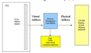
All addresses in programs are now considered "virtual". When the CPU accesses memory the virtual memory address is on the fly translated into a physical address. The MMU is a piece of hardware, nowadays mostly within the CPU but page tables are maintained by the operating system. The relocation problem is solved because all programs contain the same virtual addresses which are mapped to different physical addresses.
