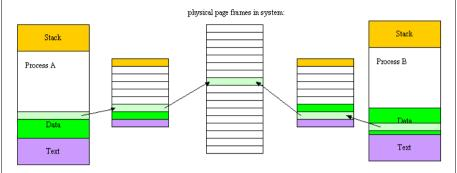
Simply by putting the same physical address into two different page table entries from different processes they can share this piece of memory. This is usually caused by both processes executing a special memory map system call. Notice that the shared memory is in different virtual memory locations in both processes.
