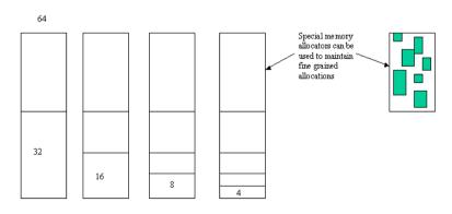
Diagram from Tanenbaum pg. 721. The buddy algorithm avoids total fragmentation of memory by merging neighbouring chunks if they become free. Allocation is by power of two only which can waste quite a bit of memory. Internal fragmentation is high.
