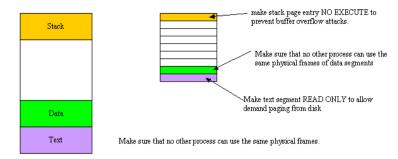
It is through the bits in the page table entries that the operating system protects a processes pages. Buffer overflows are security attacks where attack code is planted on the stack and executed there. Preventing execution in the stack segment is one way to prevent those attacks (at least partially). Most paging systems lock code (text) during execution. Self-modifying code proved to be extremely hard to program.
