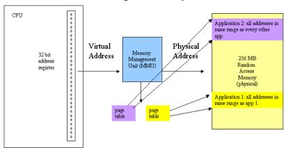
All addresses in programs are now considered "virtual". When the CPU accesses memory the virtual memory address is on the fly translated into a physical address. The MMU is a piece of hardware, nowadays mostly within the CPU but page tables are maintained by the operating system. The relocation problem is solved because all programs contain the same virtual addresses which are mapped to different physical addresses.
