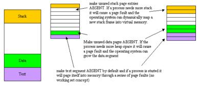
Growing segments automatically after page faults is a very elegant way to increase process resources. It has some limitations though: when does the OS know that a page fault should result in a new page allocated or the program killed because of a program execution bug? And starting a program through a series of expensive page faults is not really cheap. Better solutions use the concept of a "working set" of pages that must be present for a process to run.
