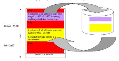
Several processes can run concurrently as long as they fit into memory. The system needs to find proper places for processes and deal with memory fragmentation due to different process sizes. If a process needs to grow and there is no free memory, some process will be "swapped" to disk to make room. Different strategies for process selection exist. Swapping can be implemented with or without separate process spaces.
