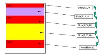
The linked list contains both program (P) and holes (H). Different lists could hold different sizes of holes so that allocation is faster.
