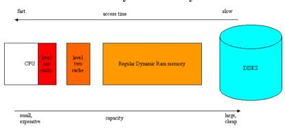
Access time and capacity are exactly reversed. To keep prices reasonable a compromise between size and speed must be met. The trick is to use caching as much as possible to keep frequently used data in the small but fast areas of the memory hierarchy. Virtual memory management allows us to treat non-Ram space like discs as memory extensions invisible to programs. This is called paging or swapping and will be explained shortly.
