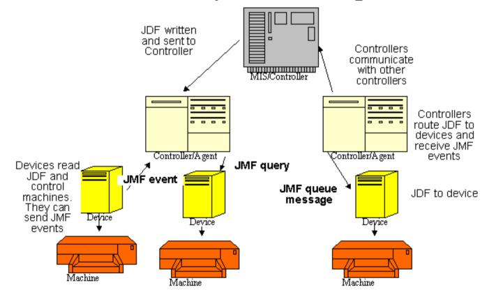
Controller, Agent and device are purely logical functions. Agents producte JDF. Controller route JDF and devices interprete and execute JDF. Devices can send events and respond to queries about their state. MIS collect this information and control the whole job. See: JDF 1.1 specification, pages 10-13
