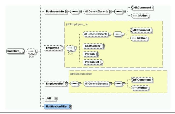
Nodeinfo elements deal with job tracking. The embedded JMF element allows the node to establish a persistent notification channel to an MIS system.
