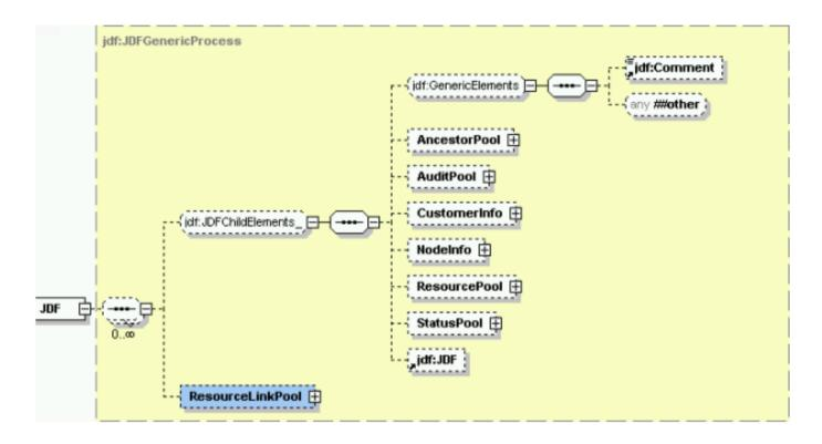
The JDF Node is the core element of JDF. It contains other core elements and can be used recursively to extend a specific JDF instance by adding more and more node elements. Rectangles with rounded corners are abstract types which cannot be direct elements of JDF instance files. Diagram generated with XMLSpy.
